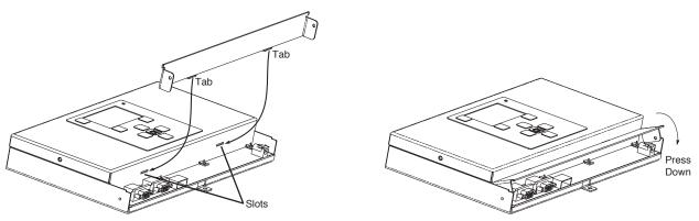
The Port Cover can be removed for access to the Initialize Button, Configuration DIP Switches, and Diagnostic LEDs. The cover is removed by gently pulling up on the front edge to disengage the snaps. Replace the cover by inserting the two tabs on the back of the cover into the slots on the processor. Gently press down on the front edge to engage the snaps.
