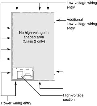
Power wiring entry (remove high-voltage cover to access)
